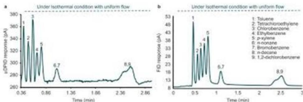
FIG. 3. Comparison of the response of the  $\mu$ DPID and the FID to 10  $\mu$ l headspace volume of C7-C10 mixture under isothermal conditions at 40 and a flow rate of  $1.33 \text{ ml min}^{-1}$  [31].
