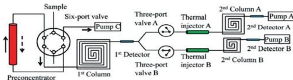
FIG. 2. The schematic diagram of chip-based multidimensional gas chromatograph: each column has separate injector and on-column optical fiber detector [2].
