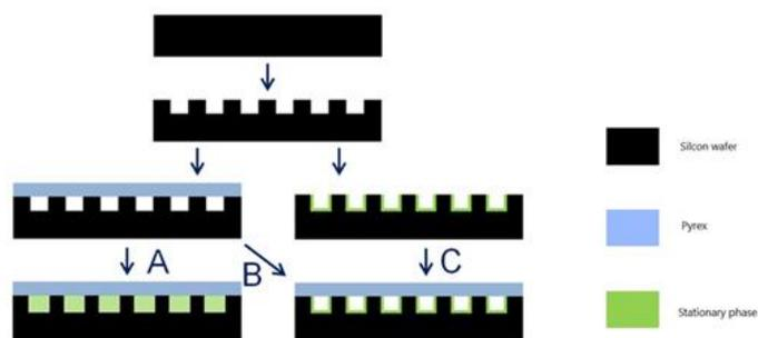
**FIG. 1. The general idea of Silicon-Pyrex microcolumns fabrication for miniaturized gas chromatographs using MEMS technology.**
