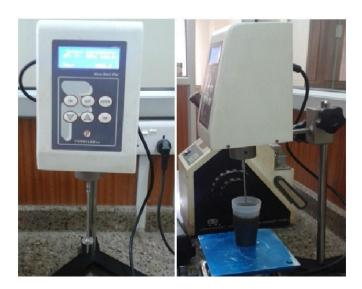
FIG. 1. Rotational Viscometer for bio-resin characterization.
