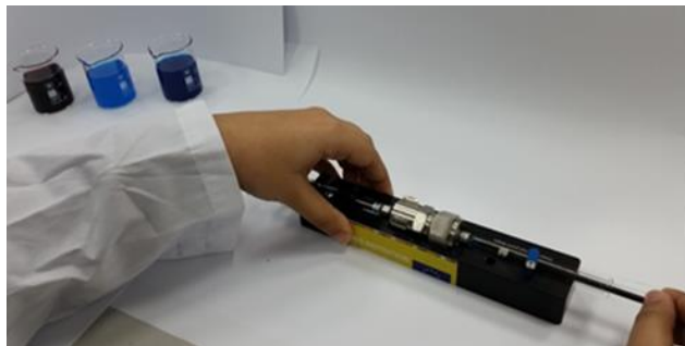
FIG. 1. Mini Extruder apparatus, passing drug loaded liposomes through its membranes [5].
