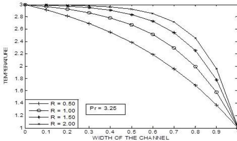
FIG. 7. Temperature profiles along the width of the channel.
