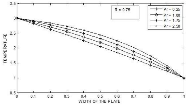
FIG. 2. Variation of temperature along the width of the channel.
