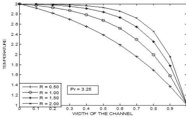
FIG. 6. Temperature profiles along the width of the channel.
