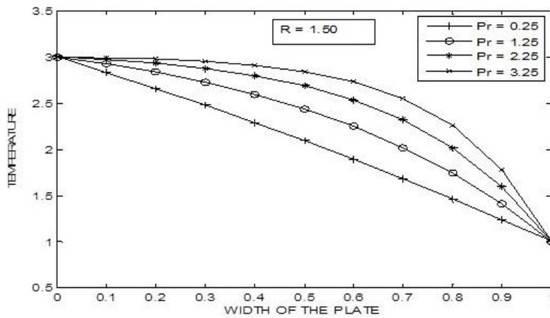
FIG. 4. Variation of temperature profiles along the width of the channel.
