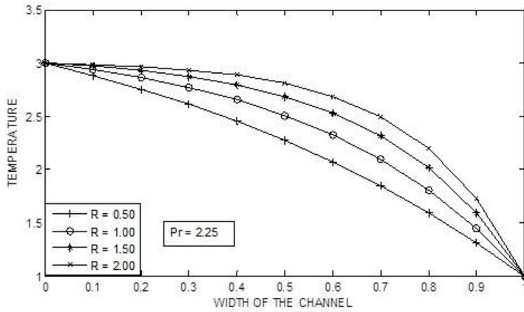
FIG. 8. Temperature profiles along the width of the channel.
