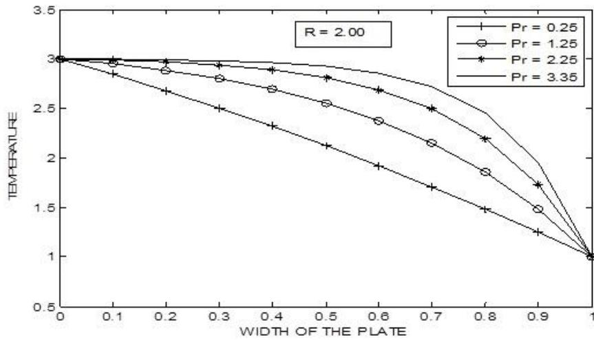
FIG. 3. Distribution of temperature profiles along the width of the channel.
