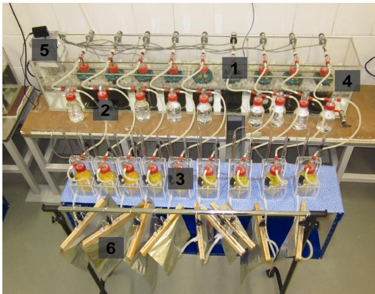
FIG. 2. Picture of one BatchLab setup including 9 units. It consists of digester tanks (1), NaOH units (2), gas drying units and gas volume sensors (gasUino) (3), tempered water bath (4), thermostat (5) and gas collection bags (6).
