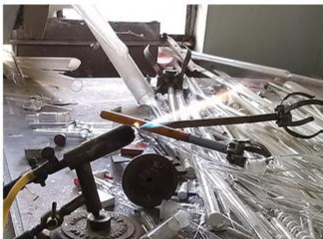
FIG. 3. Encapsulation through quartz glass blowing.
