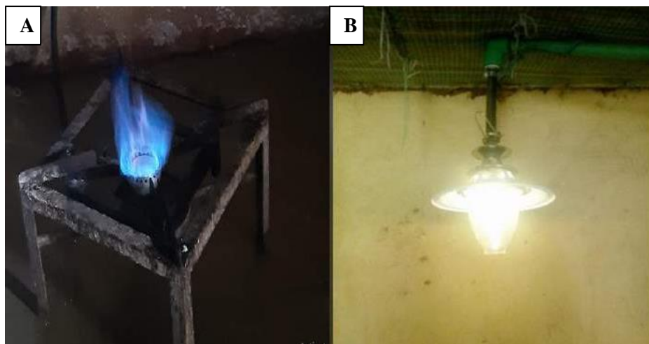
FIG. 8.A.B. Images of biogas stove and lamp installed at AGRC, Birbirsa (A) Biogas stove (B) Lamp installed
