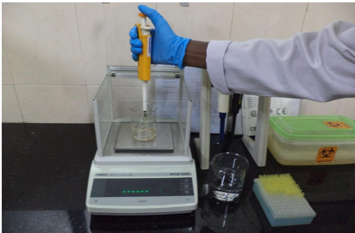
FIG. 1. Gravimetric test of pipette calibration.
