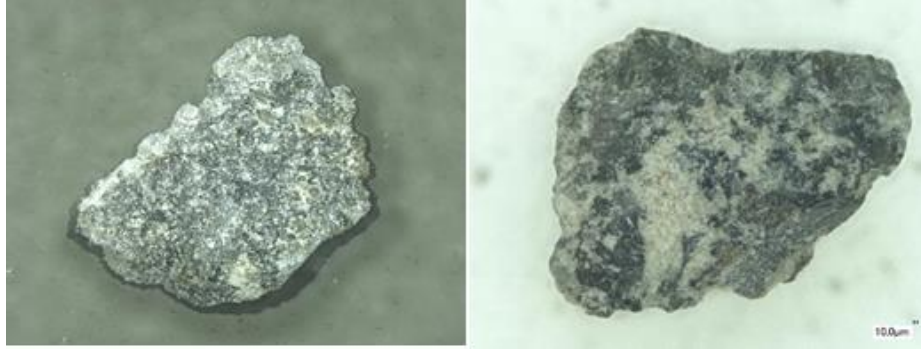
FIG. 2. Microscopic image of basalt (left) and gabbro (right) used in TUBS simulants in the range > 1000\mu\text{m}
