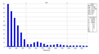
FIG. 3.6 Current harmonics (Battery-Solar Source)
