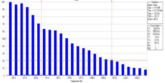
FIG. 3.1 Current harmonics (Battery Source).
