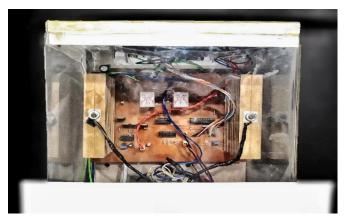
FIG. 2.2 Microcontroller connections (smart solar inverter)
