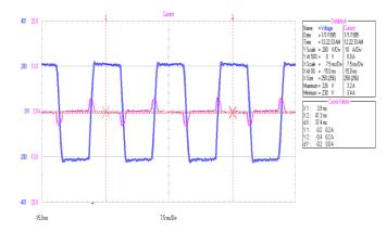
FIG. 3.5 Voltage and current waveforms (Battery-Solar Source)
