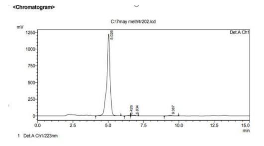
FIG. 3. The HPLC chromatogram of crude Andrographolide (NPL/AD/003).
