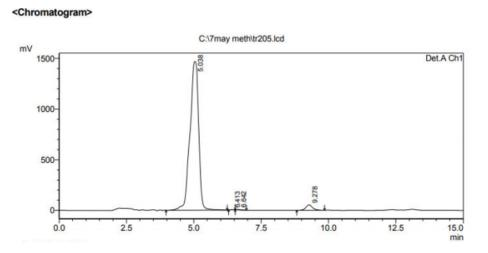
FIG. 4. The HPLC chromatogram of pure Andrographolide (BNPL/AD/006).
