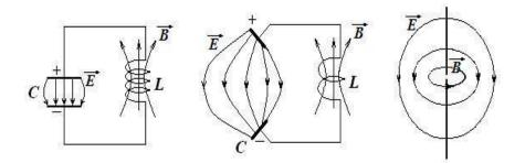
FIG. 1. Transformation of a closed electrical oscillatory circuit into the open.
