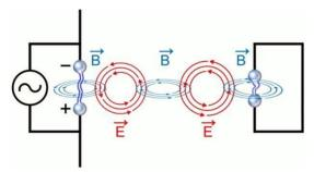
FIG. 2. The emergence of an electromagnetic wave.
