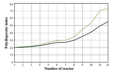
Fig. 6: Changing polydispersity index of the formed copolymer depending on the number of reactor: the dotted line – 15 hrs, the solid line – 30 hrs conducting of the process
