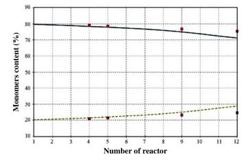
Fig. 7: Dependence of weight content of butadiene (solid line) and styrene (dotted line) from number of the reactor (points - experimental data)
