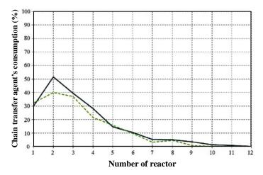
Fig. 5: Changing chain transfer agent's concentration in the reactors: the dotted line – 15 hrs, the solid line – 30 hrs conducting of the process
