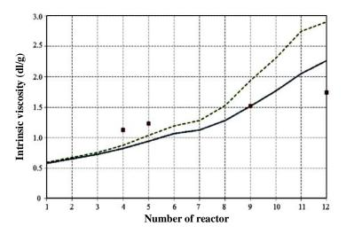
Fig. 3: The dependence of the calculated (lines) and experimental (points) intrinsic viscosity's values from reactor's number in the cascade: the dotted line – 15 hrs, the solid line – 30 hrs conducting of the process
