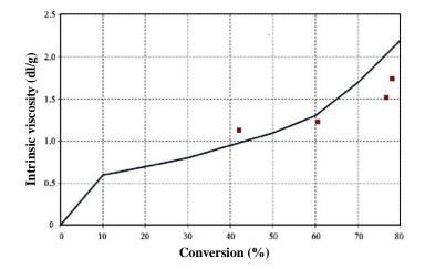
Fig. 4: The dependence of the calculated (lines) and experimental (points) intrinsic viscosity's values from conversion of monomers
