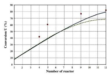
Fig. 2: The dependence of the calculated (lines) and experimental (points) conversion's values from reactor's number in the cascade: the dotted line – 15 hrs, the solid line – 30 hrs conducting of the process
