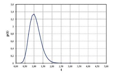
Fig. 1: Residence time distribution in the cascade of 12 reactors
