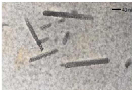
Figure 2 : HRTEM micrograph of ZnS nanocomposite nanorods.
