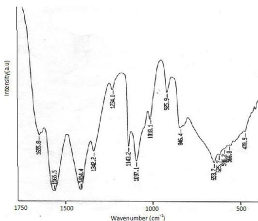
Figure 5 : FTIR spectrum of ZnS nanocomposite nanorod.
