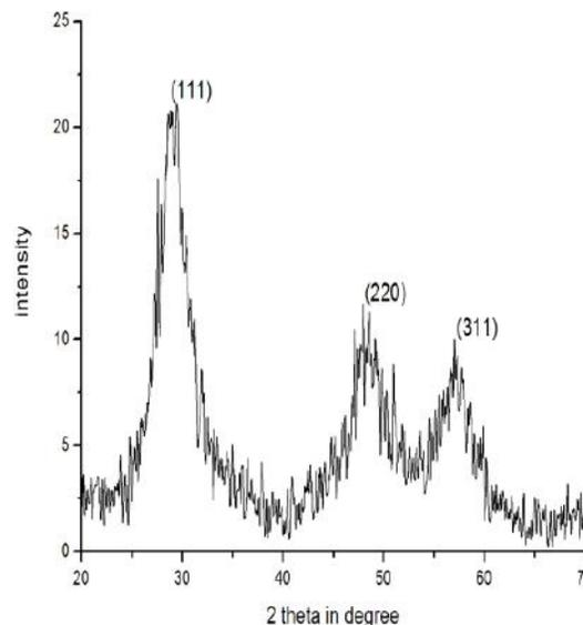
Figure 1 : XRD pattern of ZnS nanocomposite thin film
