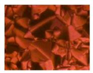
Figure 1: A typical SmB phase texture photograph observed between crossed polarizers (homeotropic alignment)
