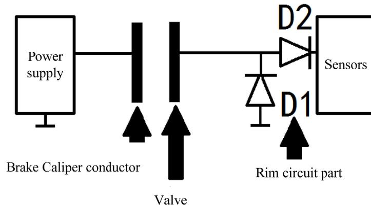
**Figure 1 : The principle of indirect TPMS figure**
