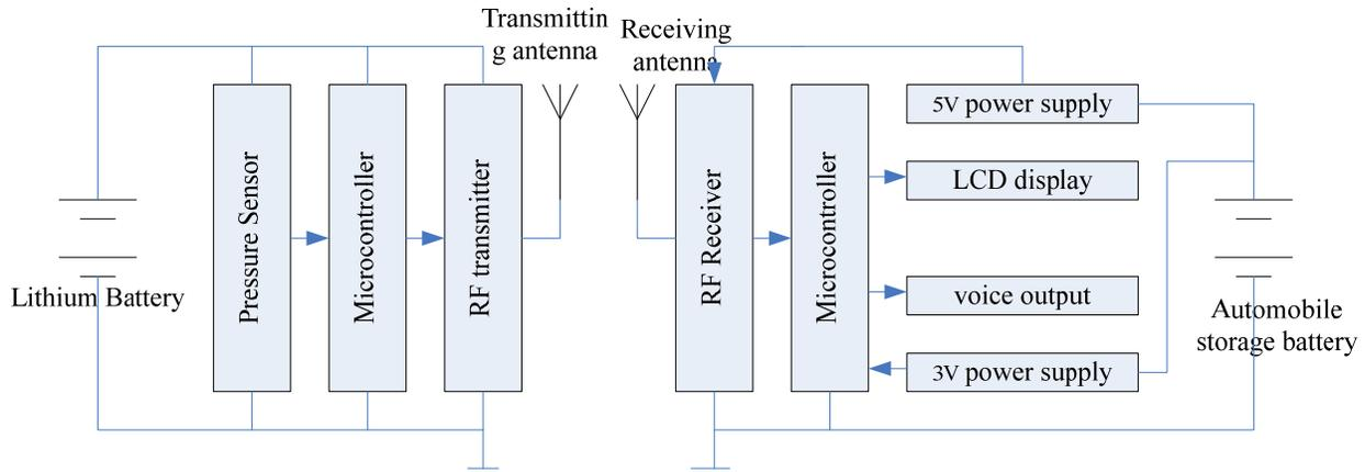
**Figure 2 : WSB - TPMS system work framework**
