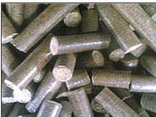
**Fig. 1: Briquettes of bio-coal**
