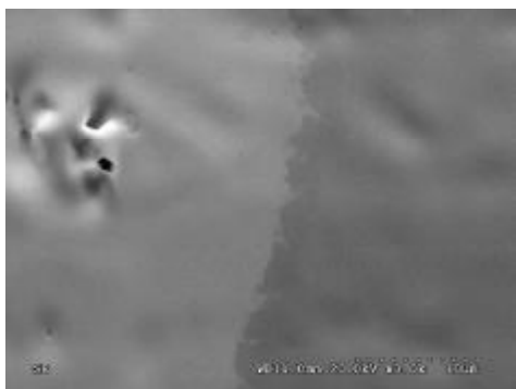
Figure 8: Scanning electron micrographs of interface of polymeric films formed on gold electrode in 0.1M HClO 4 solution from o-aminobenzoic acid
