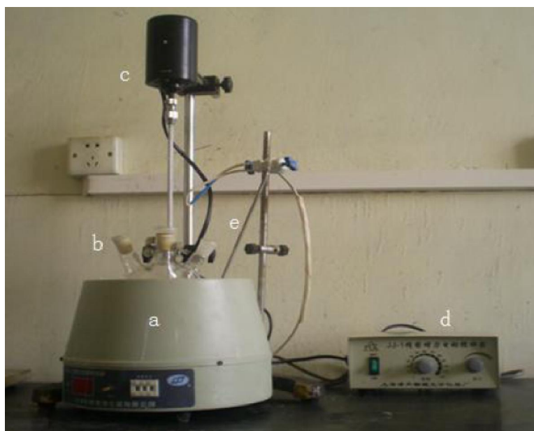
a: electric heater; b: three flask; c: agitator; d: controller; e: thermal couple
