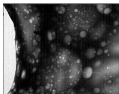
Figure 3 : TEM Micrograph of the reactive blend between epoxidized particles and epoxy resin
