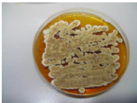
Figure 2 : Visual fungal growth on LDPE/ corn starch blend after 84th day's incubation.
