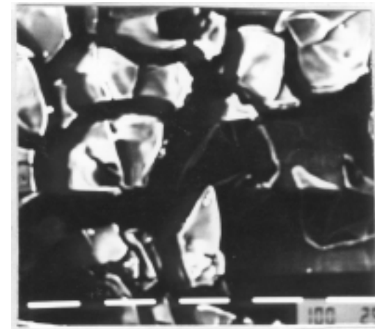
Figure 7a: SEM micrograph of the formed siliconized film at 675°C & 150 X.
