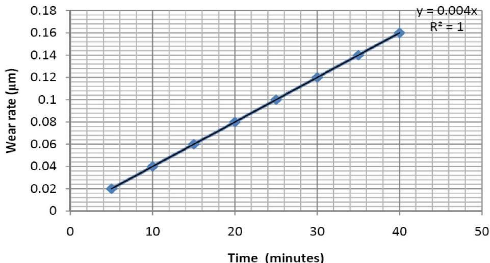
Figure 7 : Time vs. wear for the OEM brake lining
