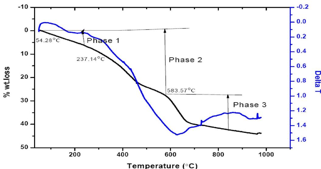
Figure 3 : TGA/DTA results of the purchased OEM friction lining material
