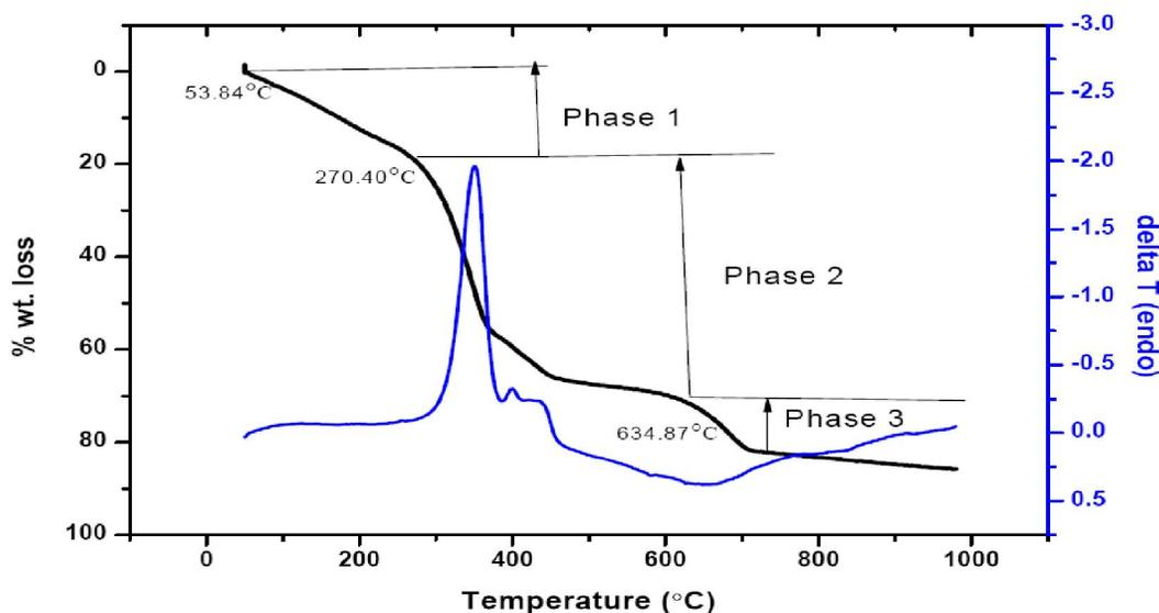
Figure 2 : TGA/DTA results of the produced PKS based friction lining material
