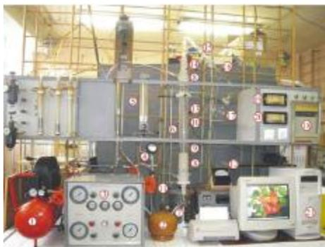
**Figure 2 :** Laboratory installation for combustion of raw rice husks in fluidized bed reactor: 1-air compressor *Black and Decker*, 2- tank for liquid petroleum gas, 3-distributor for gases, 4-manometer, 5-air Rota meter, 6-quartz fluidized bed reactor, 7-gas burner, 8-asbestos insulator, 9-porous quartz diaphragm, 10-electrical heater, 11-electrical transformer, 12-voltmeter, 13, 14 15-thermo couples, 16-economizer, 17-separator, 18-temperature recorder, 19, 20-thermo regulators, 21-PC
