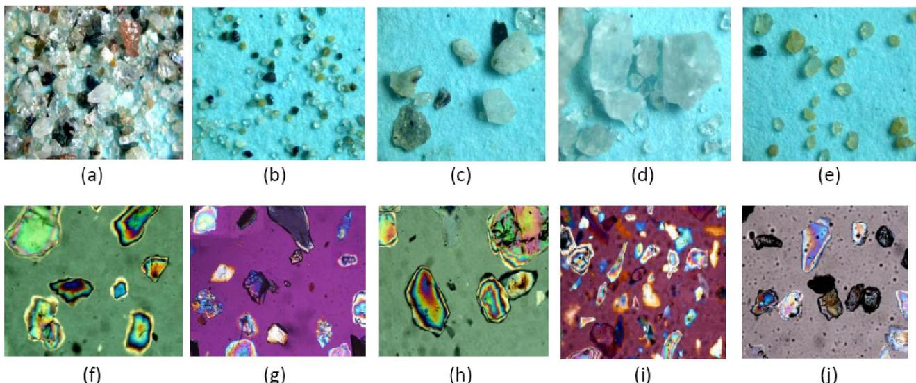
Figure 2: Stereo-microscopic view of (a) Dalia, (b) Kuakata, (c) Patgram, (d) Bipinganj and (e) Sylhet sand and Polarizing microscopic view of (f) Dalia, (g) Kuakata (crossed polarized), (h) Patgram, (i) Bipinganj (crossed polarized) and (j) Sylhet (plane-polarized)
