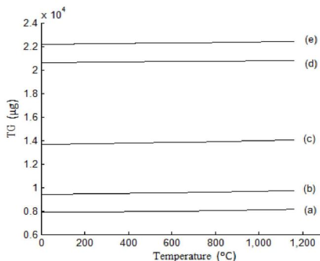
Figure 6 : Thermogravimetric analysis of (a) Sylhet, (b) Bipinganj, (c) Dalia, (d) Patgram and (e) Kuakata sand
