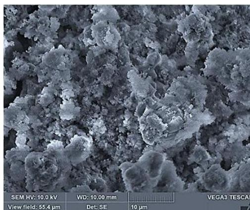
FIG. 6. SEM showing agglomerates of elaborated pseudoboehmite particles.
