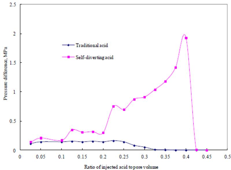
**Figure 3: Experimental results of injection pressure with different acid**
