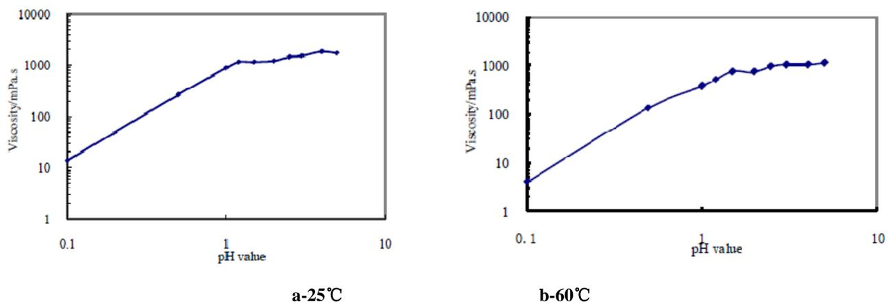
Figure 1: Relationship between viscosity and residual acid concentration under 25 °C and 60 °C
