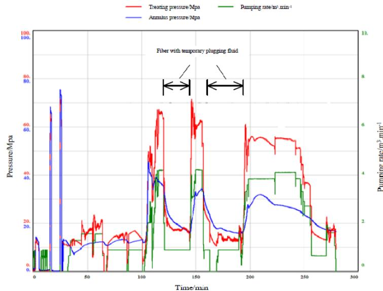
**Figure 7: Acid-fracturing curve temporary plugged by clean self-diverting acid and fiber of Well A**
