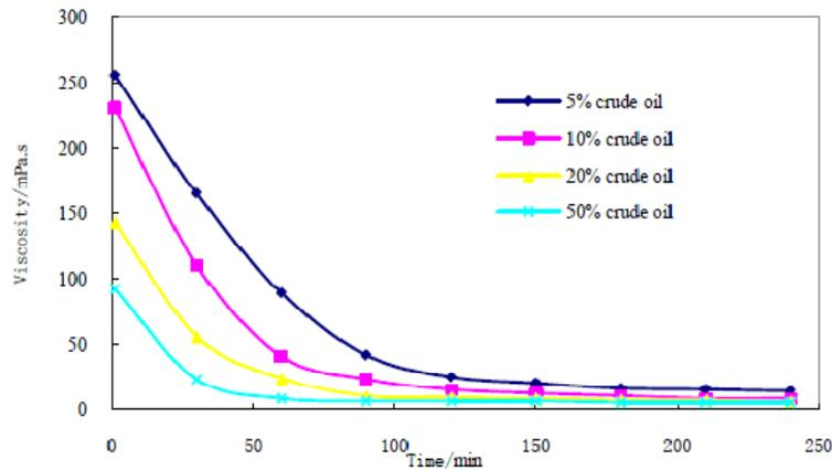
Figure 4 : Variation of residual acid viscosity after mixed with different quantity of crude oil
