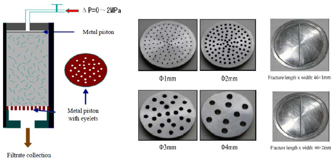
Figure 5: API leakage apparatus and different types of metal pistons
