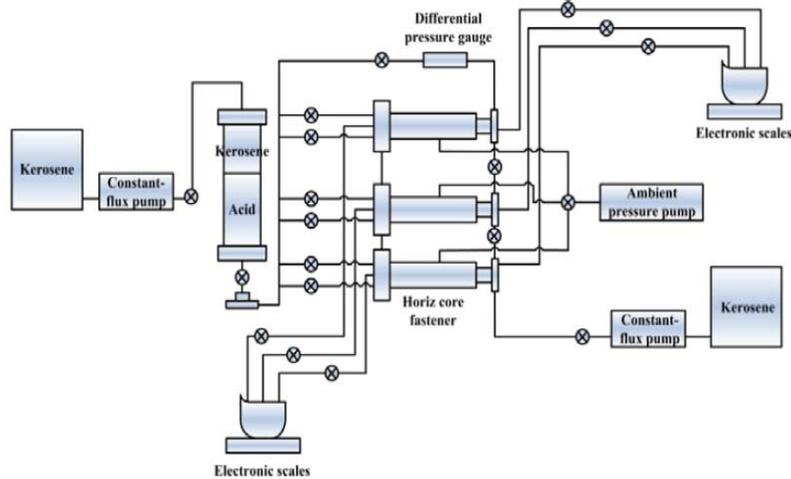
**Figure 2 : Experimental equipment of self-diverting acid flowing in core**
