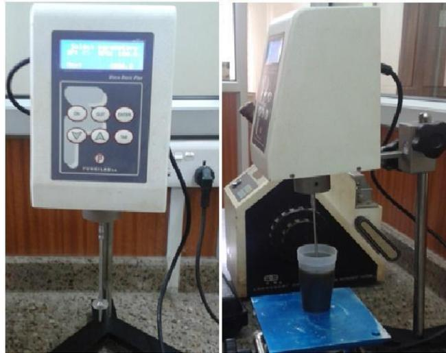
FIG. 1. Rotational Viscometer for bio-resin characterization.
