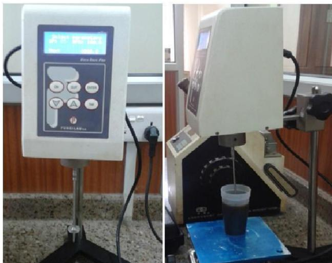
FIG. 1. Rotational Viscometer for bio-resin characterization.
