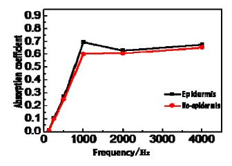
Figure 5 : The affection of epidermis on absorption characteristics **RESULTS**
