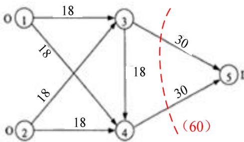
Figure 2 : The example network of calculation (The numbers in the figure represent the traffic capacity of the road sections and node numbers)
