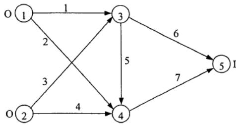
Figure 1 : The example network of calculation (The numbers in the figure represent the road sections and node numbers)
