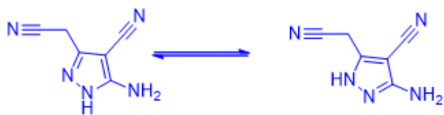
FIG.5. Tautomeric forms of the 5-amino-3-(cyanomethyl)-1H-pyrazole-4-yl cyanide compound.
