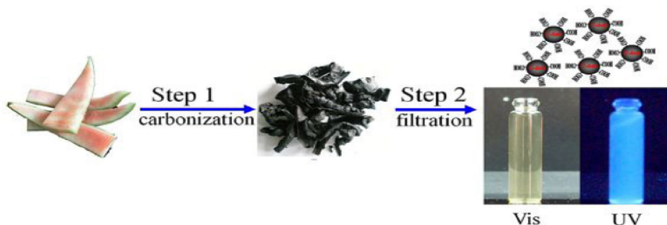
Figure 5 : The synthesis of water-soluble fluorescent CDs from watermelon peel
