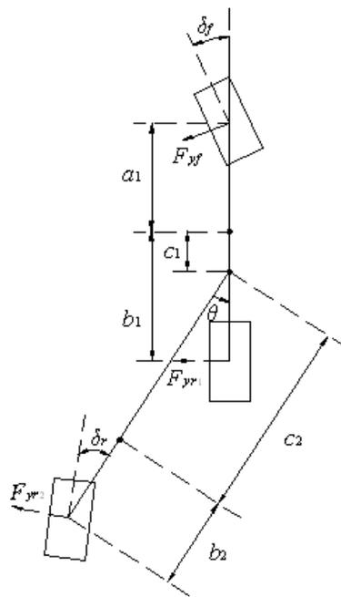
Figure 1 : Schematic diagram of 4WS tractor-semitrailer
