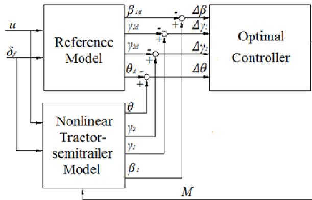
**Figure 2 : Schematic diagram of the optimal controller principle**
