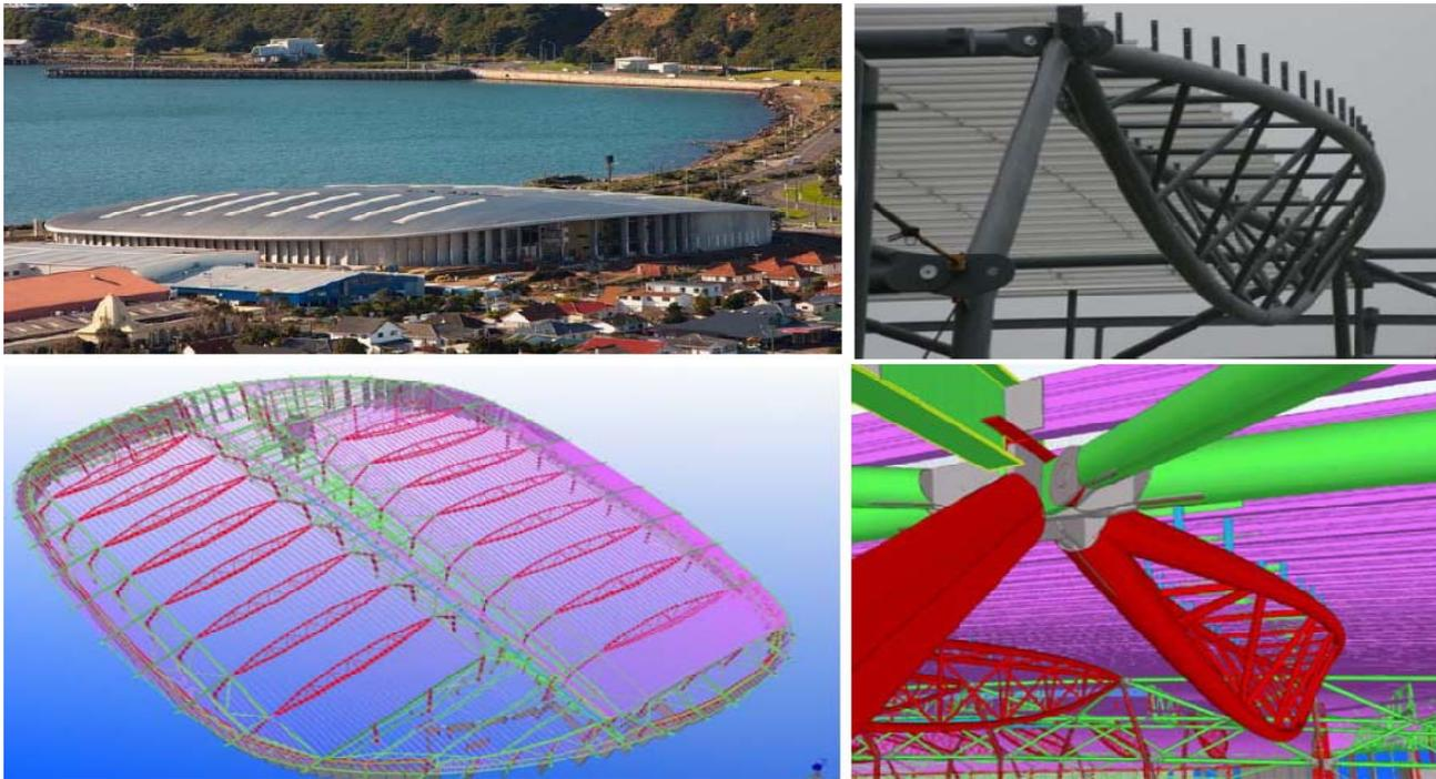
**Figure 4 : BIM can provide comprehensive and detailed three-dimensional virtual model of the building**
