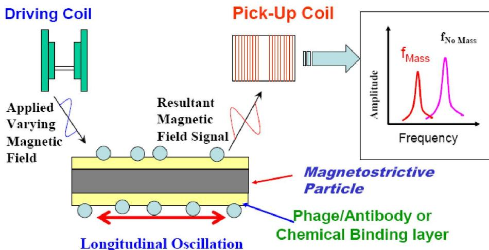
Figure 1 : Schematic illustration of the wireless nature of the magnetostrictive biosensors
