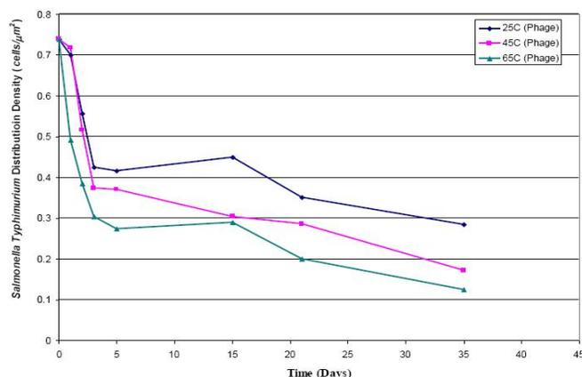
Figure 2 : The longevity of Magnetostrictive biosensors at different temperatures
