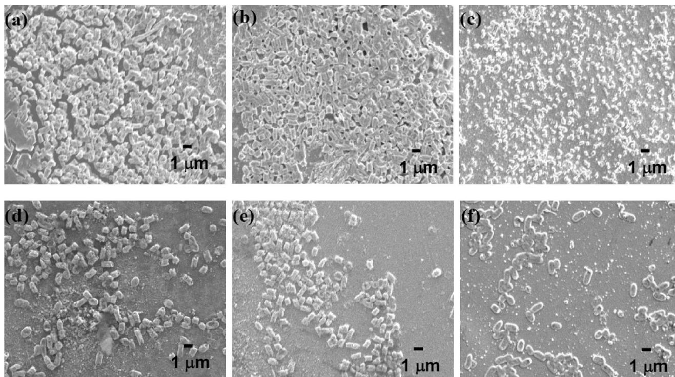
**Figure 3 :** Typical SEM images of *S. typhimurium* bacterium bound to the phage immobilized biosensor surface after different duration at different temperatures (a) to (c) Day 0 at 25°C, 45°C, 65°C, respectively, (d) and (f) Day 30 at 25°C, 45°C, 65°C, respectively
