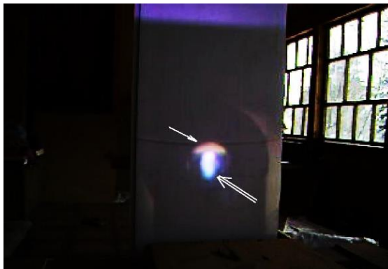
FIG. 2. A frame from the video recording, containing an image of a light spot when sodium nitrate was not added to the discharge gap. The single arrow points to the red-orange spot, the double arrow points to the blue spot.
