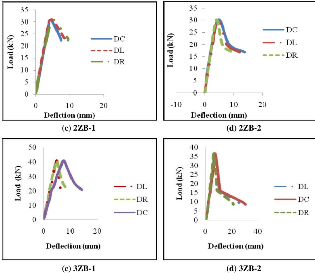
**Fig. 4: Load versus deflection curves for the test specimens**
