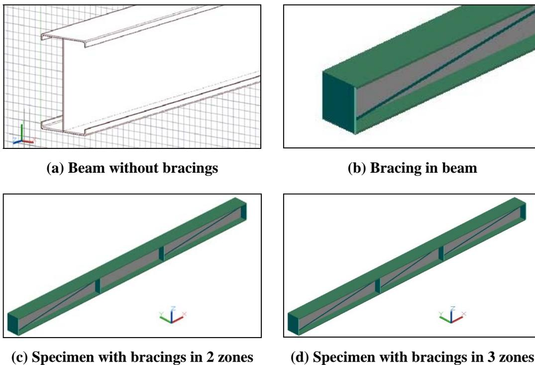
Fig. 1: Details of beam specifications
