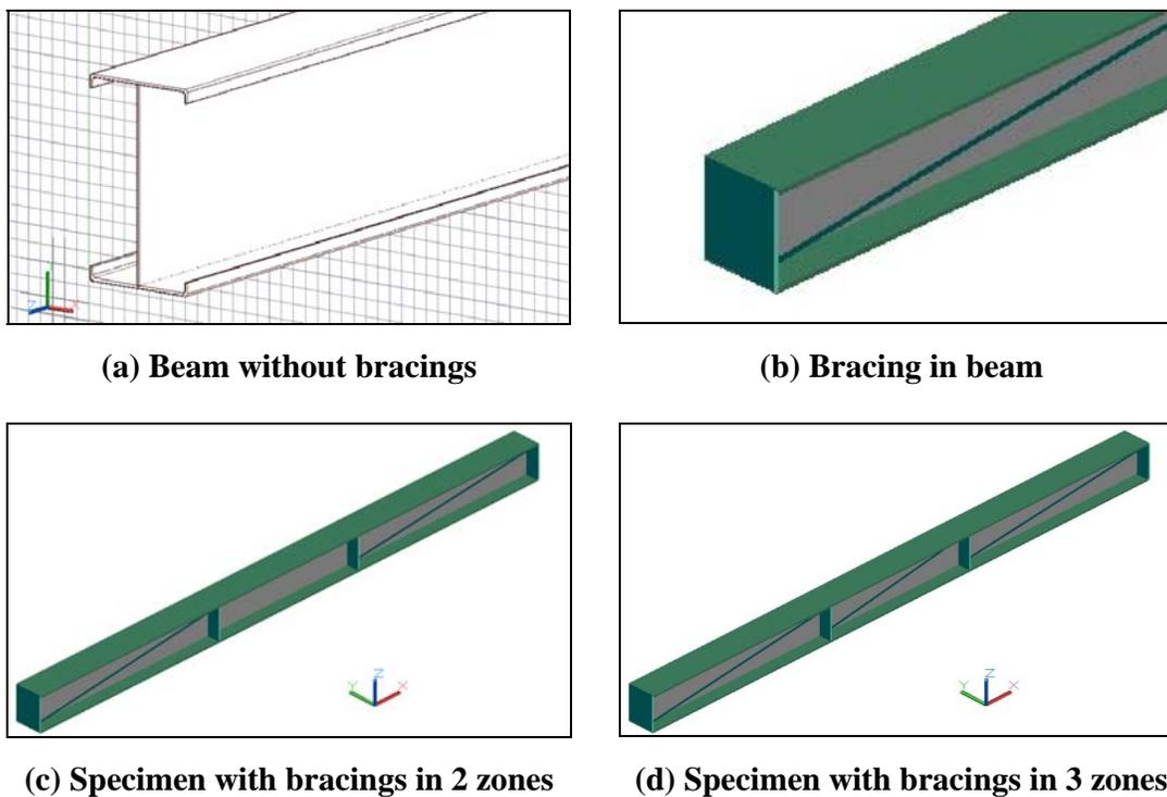
Fig. 1: Details of beam specifications
