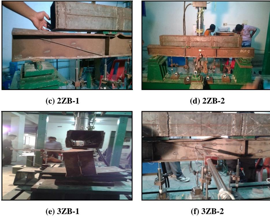
Fig. 3: Failure pattern of the test specimens
