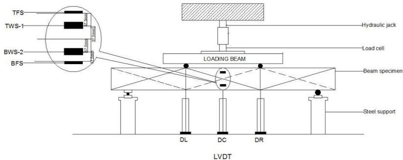
**Fig. 2 Position of LVDTs and strain gauges**
