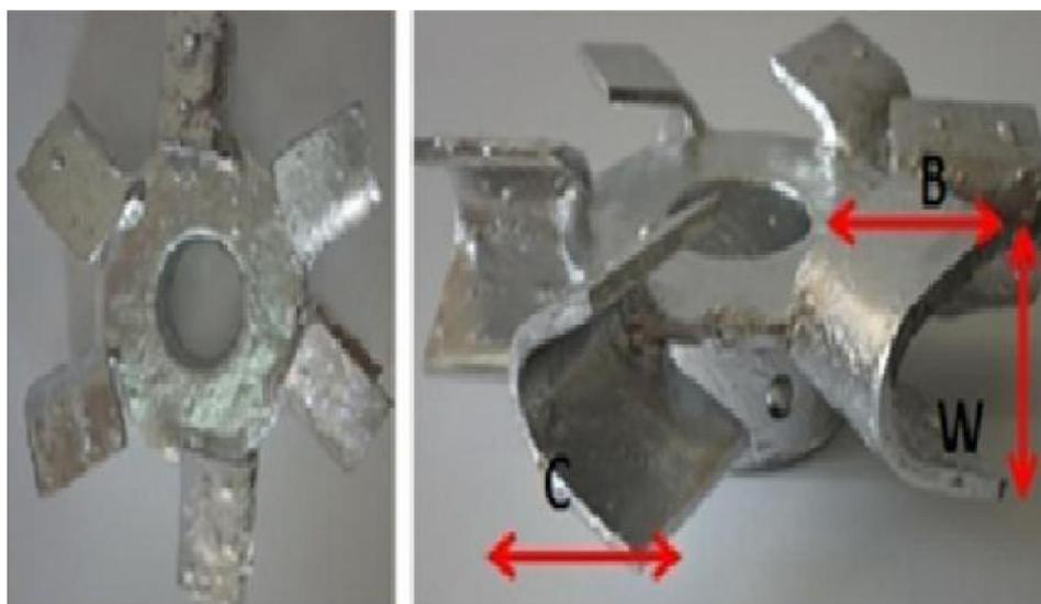
Figure 2 : Shape of a concave impeller
