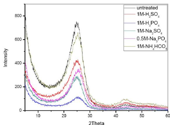
**Figure 8 : The XRD curves of carbon fibers treated in different electrolytes**
