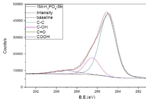
Figure 4 : C1s peak separation of carbon fiber treated in 1M  $\text{H}_3\text{PO}_4$  for 5h
