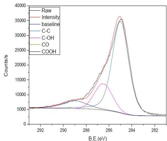
Figure 3 : C1s peak separation of carbon fiber treated in 1M  $\text{H}_2\text{SO}_4$  for 5h
