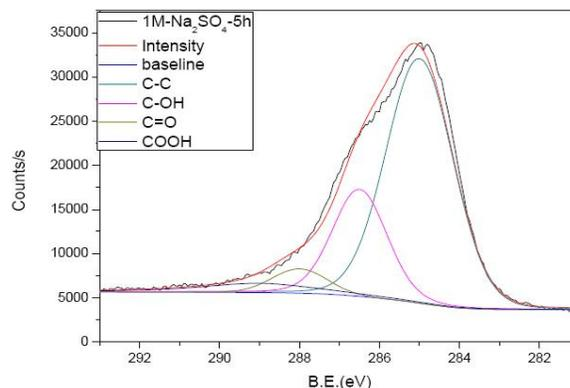
Figure 5 : C1s peak separation of carbon fiber treated in 1M  $\text{Na}_2\text{SO}_4$  for 5h
