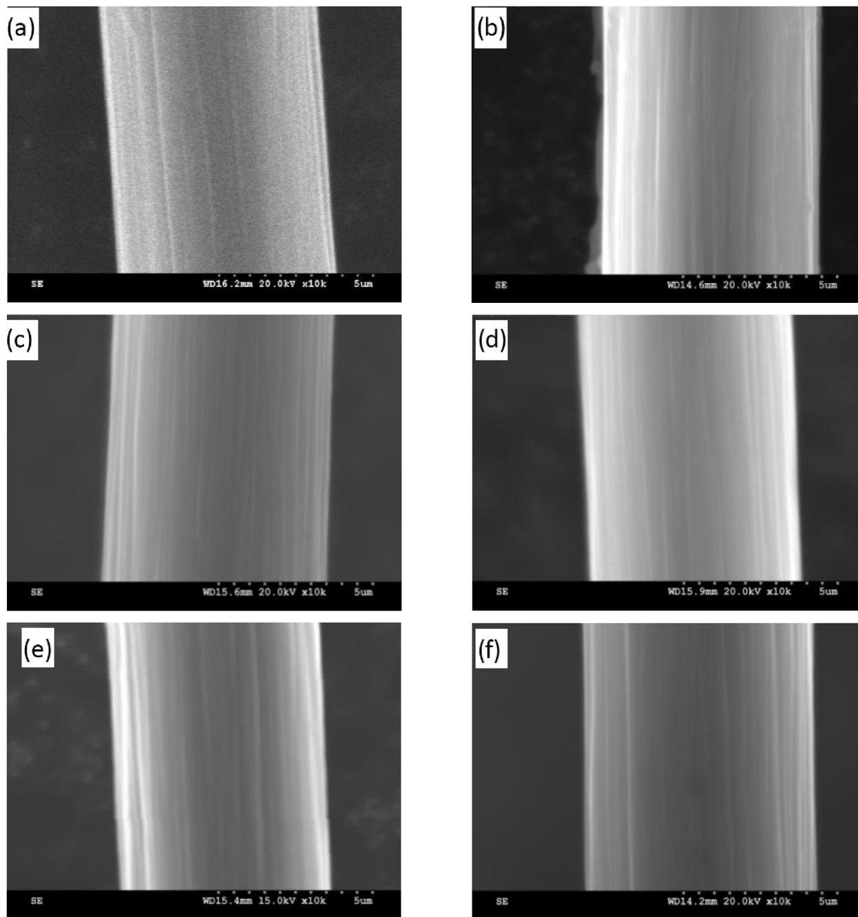
Figure 1 : The SEM photographs of carbon fibers untreated and treated (a) untreated (b) in 1M-H<sub>2</sub>SO<sub>4</sub> (c) in 1M-H<sub>3</sub>PO<sub>4</sub> (d) in 1M-Na<sub>2</sub>SO<sub>4</sub> (e) in 0.5M-Na<sub>3</sub>PO<sub>4</sub> (f) in 1M-NH<sub>4</sub>HCO<sub>3</sub>
