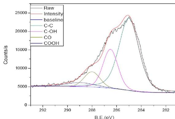
Figure 6 : C1s peak separation of carbon fiber treated in 0.5M  $\text{Na}_3\text{PO}_4$  for 5h
