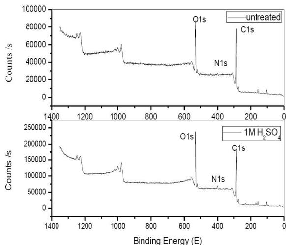
Figure 2 : Full XPS spectrum of the untreated and treated carbon fibers in 1M  $\text{H}_2\text{SO}_4$  for 5h
