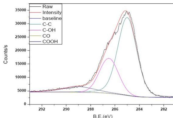
Figure 7 : C1s peak separation of carbon fiber treated in 1M  $\text{NH}_4\text{HCO}_3$  for 5h
