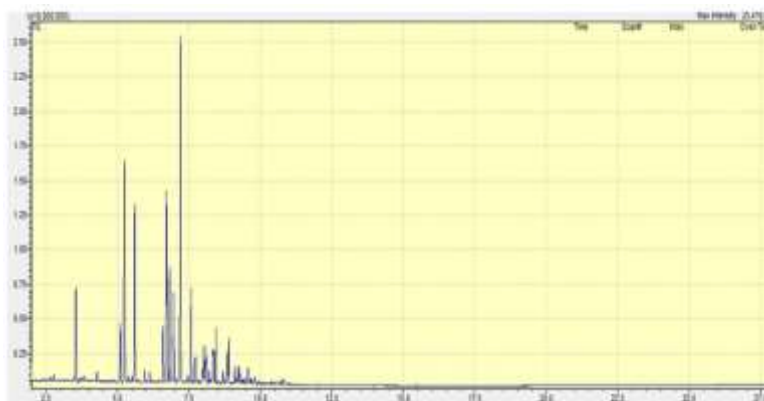
FIG. 18. TIC for petrol standard that was used in carrying out this study.
