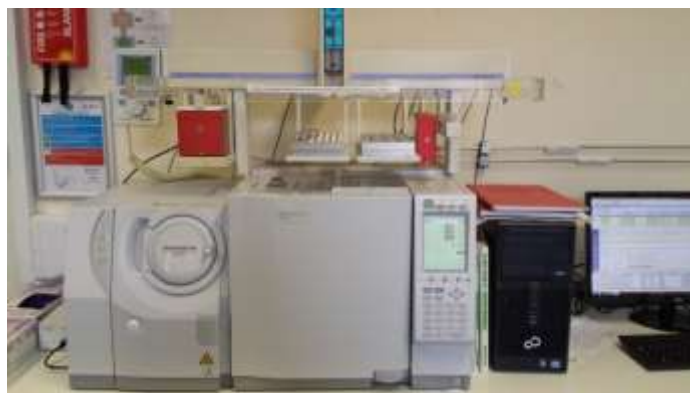
FIG. 6. Shimadzu GCMS-QP2010 SE Plus gas chromatography mass spectrometer.
