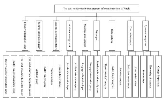
Figure 3 System module structure graph
