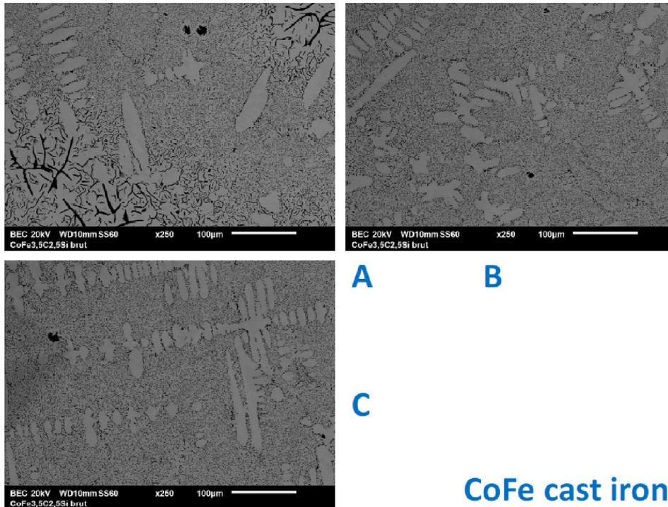
Figure 7 : Microstructure of the “CoFe” cast iron as observed with the SEM (BSE mode) in three distinct zones (“A,” B” and “C”)
