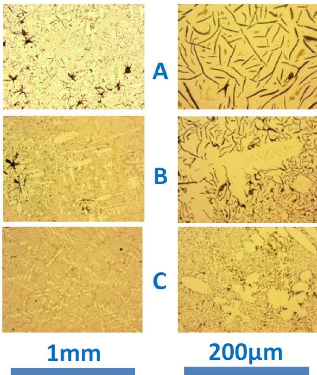
Figure 2 : Matrix structure (after Nital etching) of the "CoFe" cast iron as observed at two magnifications in three distinct zones ("A," "B" and "C")
