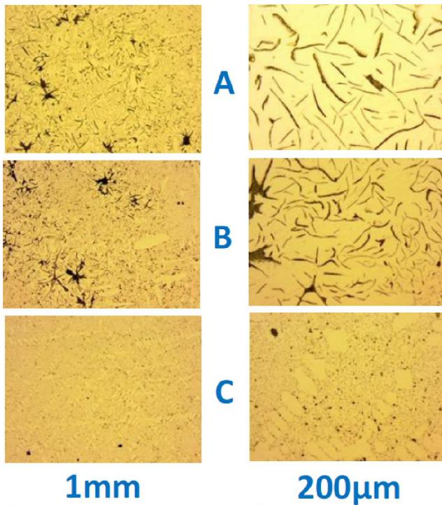
Figure 1 : Graphite structure (without etching) of the "CoFe" cast iron as observed at two magnifications in three distinct zones ("A," "B" and "C")
