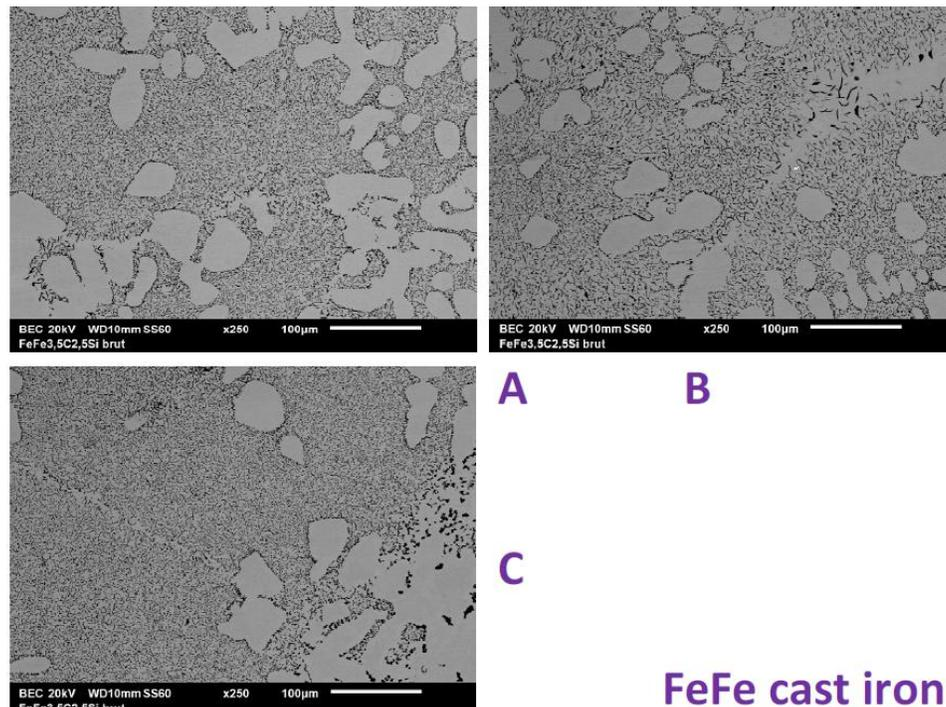
Figure 9 : Microstructure of the “FeFe” cast iron as observed with the SEM (BSE mode) in three distinct zones (“A,” “B” and “C”)
