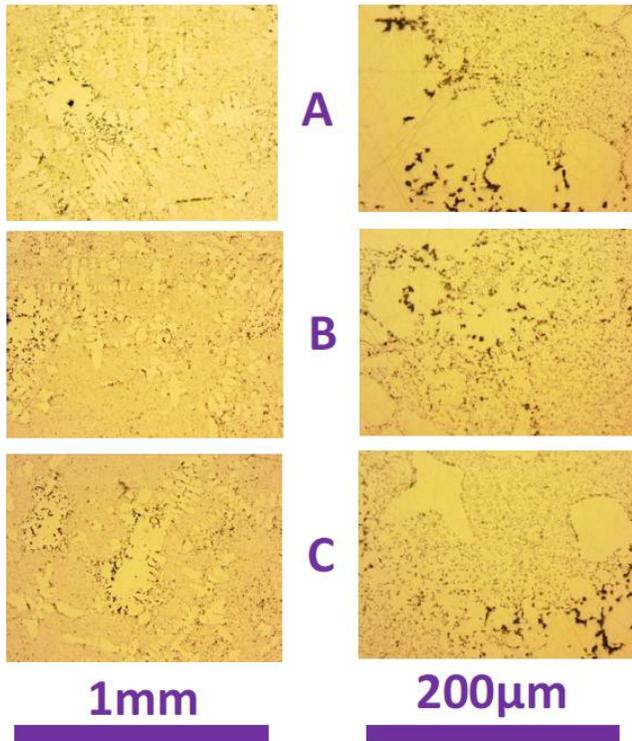
Figure 5 : Graphite structure (without etching) of the “FeFe” cast iron as observed at two magnifications in three distinct zones (“A,” B” and “C”)
