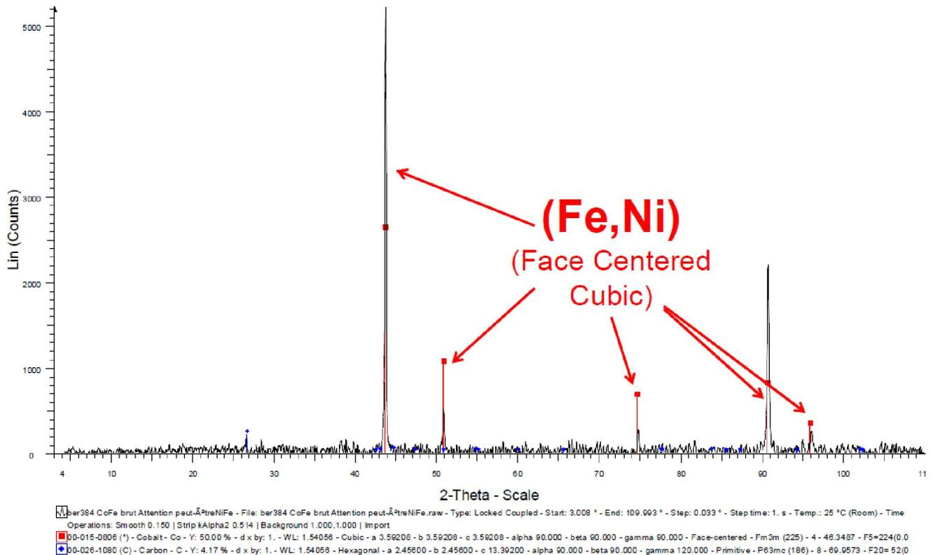
Figure 11 : X-Ray Diffractogram obtained on the "NiFe" cast iron
