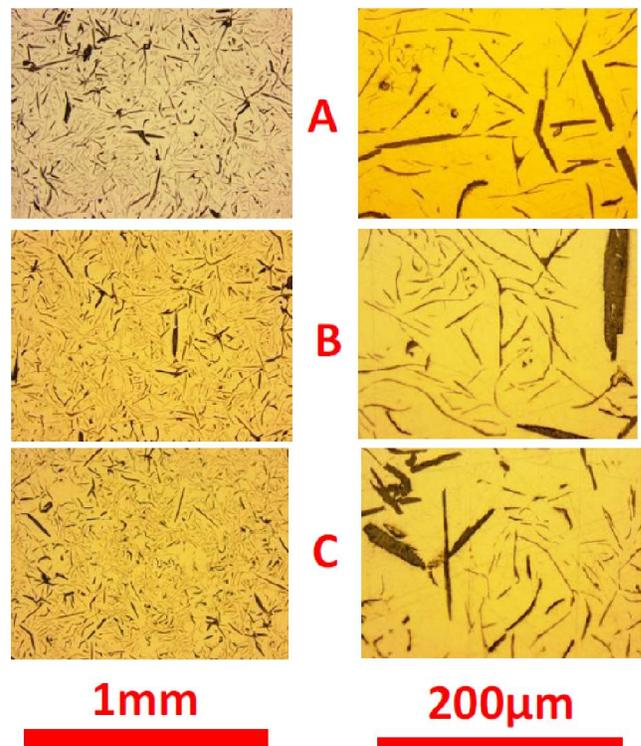
Figure 3 : Graphite structure (without etching) of the "NiFe" cast iron as observed at two magnifications in three distinct zones ("A," "B" and "C")
