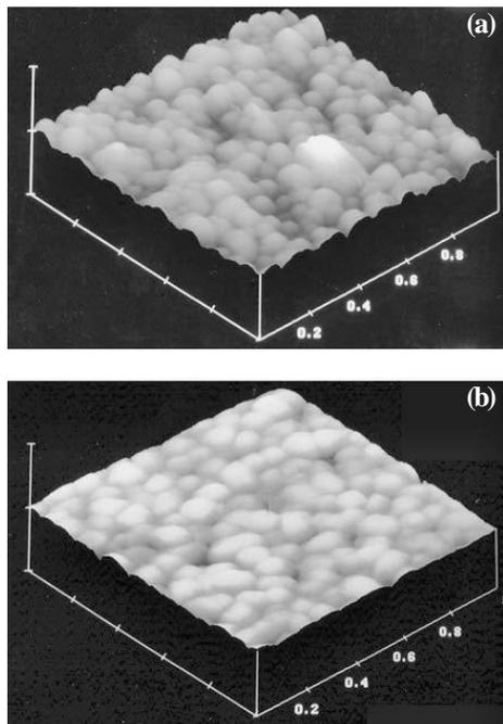
**Figure 1 :** AFM images of (a) thin film deposited from  $\text{LiCoO}_2$  pure target, and (b) thin film deposited from  $\text{LiCoO}_2$  target with 15%  $\text{Li}_2\text{O}$ .
