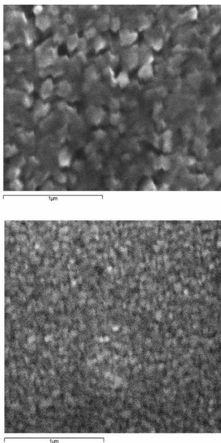
**Figure 4 :** SEM images of  $\text{LiCoO}_2$  thin films deposited at different substrate temperatures in  $p\text{O}_2 = 100 \text{ mTorr}$ .
