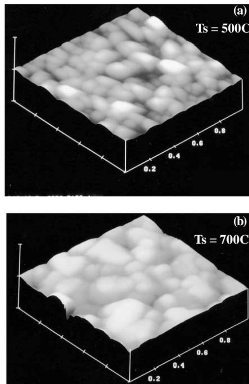
**Figure 2 :** AFM images of  $\text{LiCoO}_2$  thin films deposited at different substrate temperatures in  $p\text{O}_2 = 100$  mTorr.
