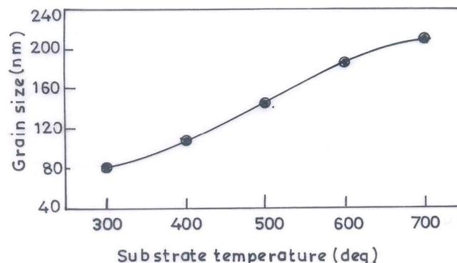
**Figure 3 :** Variation of grain size of  $\text{LiCoO}_2$  thin films with substrate temperature.
