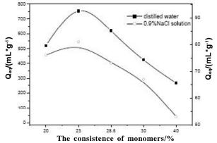
Figure 1 : Water content of copolymer with various monomer concentrations
