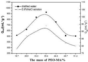
Figure 4 : Water content of copolymer with various PEGMA ratios
