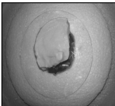
Fig. 1: Picture of soap prepared by mixing Jatropha, Castor, Mahua oil and sodium silicate
