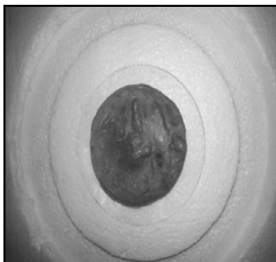
Fig. 2: Picture of soap prepared by mixing Jatropha, Castor, Mahua oil and filler (Sodium silicate) with red color and fragrance
