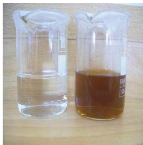
Figure 1 : Solution of silver nitrate (1 mM) before (left) and after (right) addition of seed extract solutions.
