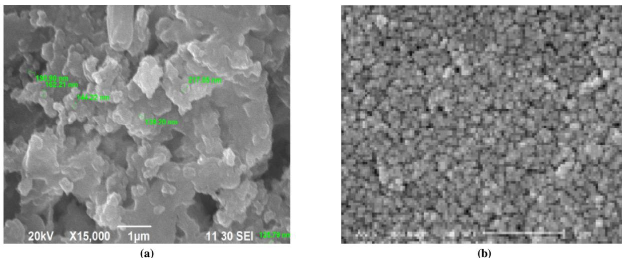
Figure 5 : SEM analysis of (a) pure and (b) synthesized silver NPs
