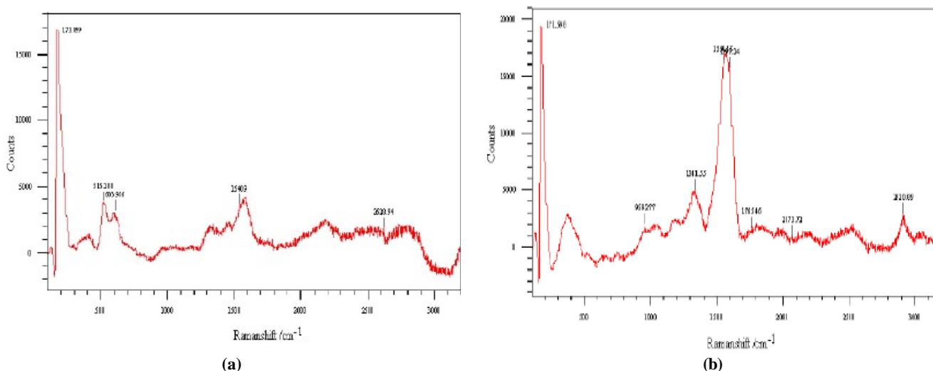
Figure 4 : FT-Raman spectra of (a) pure and (b) synthesized silver NPs
