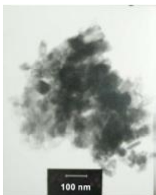
Figure 4: TEM photograph of n-Ni at 38 K
