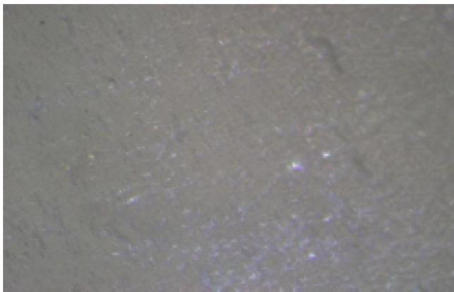
Figure 16 : (a) Pure epoxy sample at 100X magnification before wear
