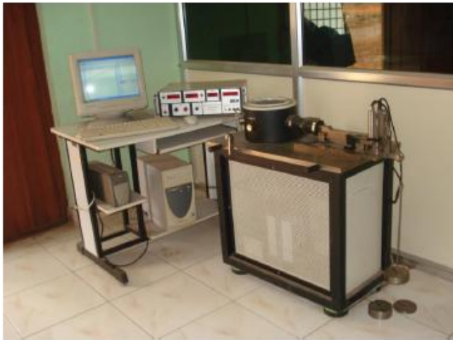
Figure 12 : Pin-on-disk set-up (DuCOM, TR-20-M26)
