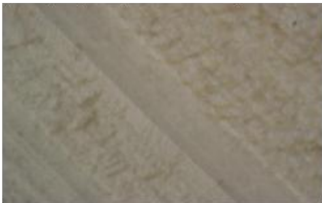
Figure 16 : (b) Pure epoxy sample at 100X magnification after 3.62 km wear distance travel
