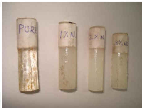
Figure 4 : Wear specimens (pure and 1,2,3wt% reinforced nano silica)
