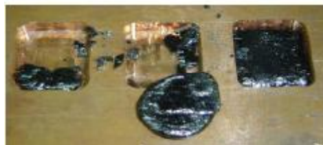
Figure 1: The as-quenched glassy plates of \text{Bi}_2\text{Sr}_2\text{Ca}_{x-1}\text{Cu}_x\text{O}_{6+\delta} ( x=1, 2, and 3 )
