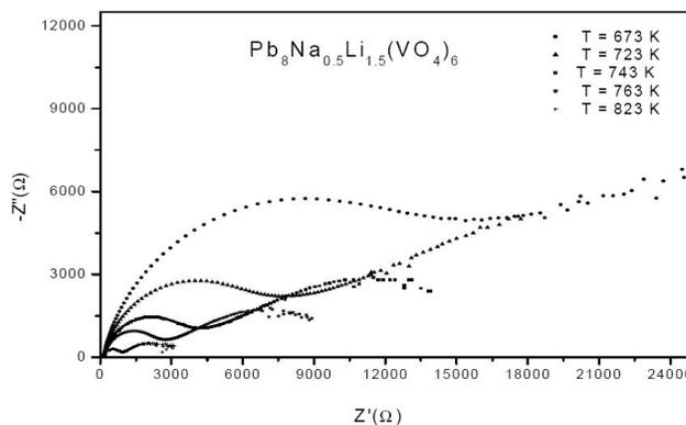
Figure 3 : Typical complex impedance diagram of  $\text{Pb}_8\text{Na}_{0.5}\text{Li}_{1.5}(\text{VO}_4)_6$ .
