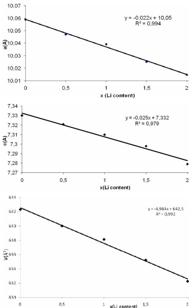
Figure 1 : Unit cell parameters variations versus Li content ( $x$ ) of  $\text{Pb}_8\text{Na}_{2-x}\text{Li}_x(\text{VO}_4)_6$  apatites
